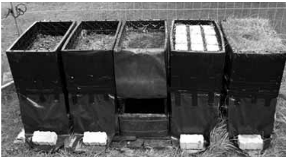
Figure 1: Experimental stormwater detention systems
